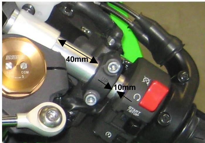
Adjust clip ons by turning the Match clamps on the slider tubes, then tighten the bolts M6x25 with 10Nm (7.31lbf ft). Now drill the bores for the controls and fix them finally. The left grip should be installed with glue.
