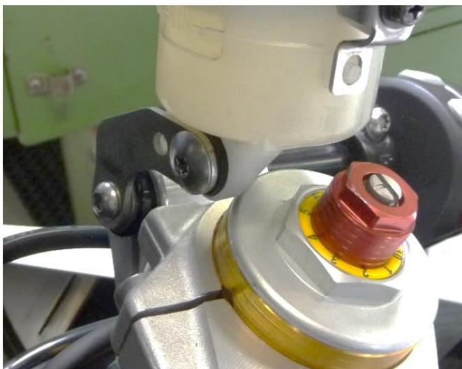
Attach the supplied bracket on the brake fluid container with the original screw.
