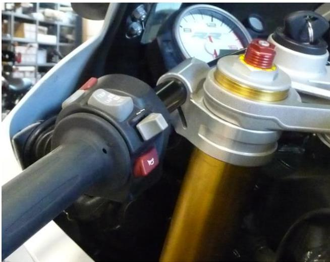
Align Speed Match clamps with bolts M6x25mm close below the top yoke.
