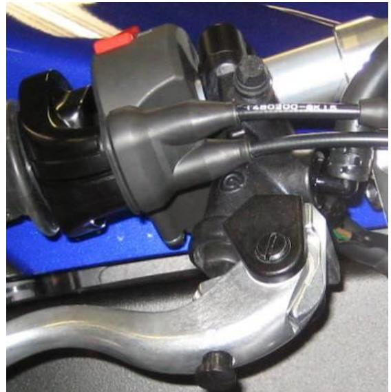
**Brake hose (2):** Mount attached brake hoses (72cm right & 74cm left) with new seal rings. The 45° fittings need to be mounted on the master brake cylinder. Mind the mounting instructions that are delivered with the brake hose. Mount right hose with rubberized clamp and M6 x 12 on the original mounting device and fix left hose with small cable tie as shown. Fix both hoses on the right slider tube with big cable tie as shown.
