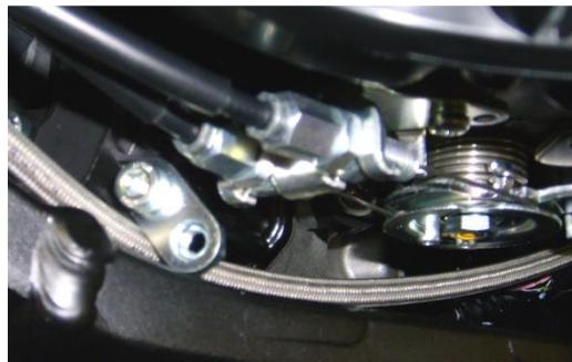
**Wiring harness (5&6):** Loose Harnesses out of guiding and Route harnesses tension free behind the slider tubes on both sides.
