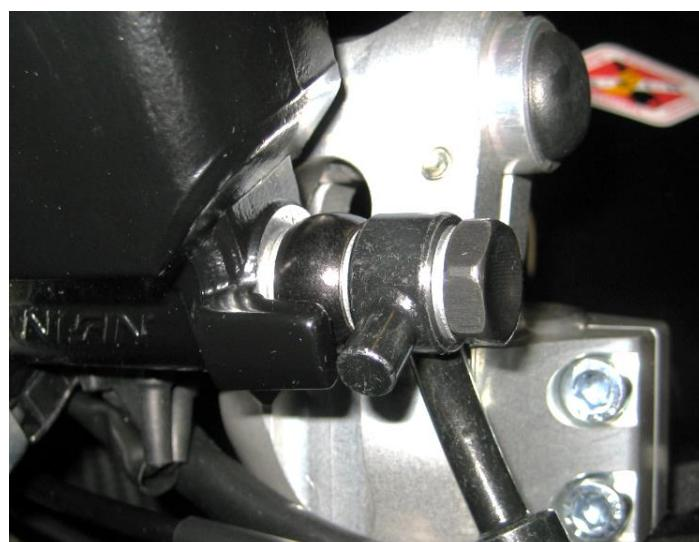
Catch brake fluid with a proper medium.
