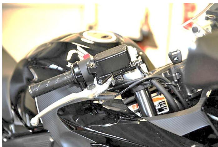
Throttle cable: carry the throttle cables below the front brake lever.
