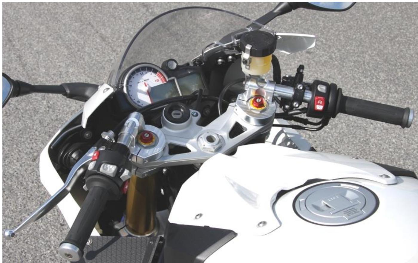
If not otherwise mentioned in text or pictures, the following tightening torques are recommended: M5 = 5Nm/3.7lbf ft; M6 = 10Nm/7.4lbf ft; M8 = 20Nm/14.8lbf ft.
