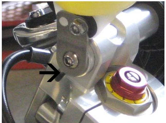
Adjust clip on by turning the Match clamps on the slider tubes, then tighten the clamping bolts finally.
