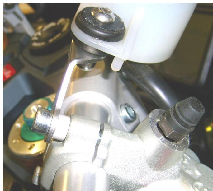
**Clutch hose:** Routing remains unchanged. Fit left reservoir as shown using mounting assy with P/N 156A015.1.
