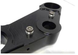
Fit the steering stop limiters, consisting of bolts (03), and bevel bushings (04), on the bottom yoke (02).
