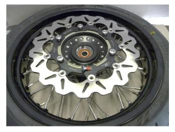
Dismantle the original brake disc. If using by LSL supplied brake disc (Art.Nr: 239T038), Galfer320mm, use distance-ring (06). If using distance-ring (06) it is necessary to use M8 x 23mm (07) for safe installation on the hub.
