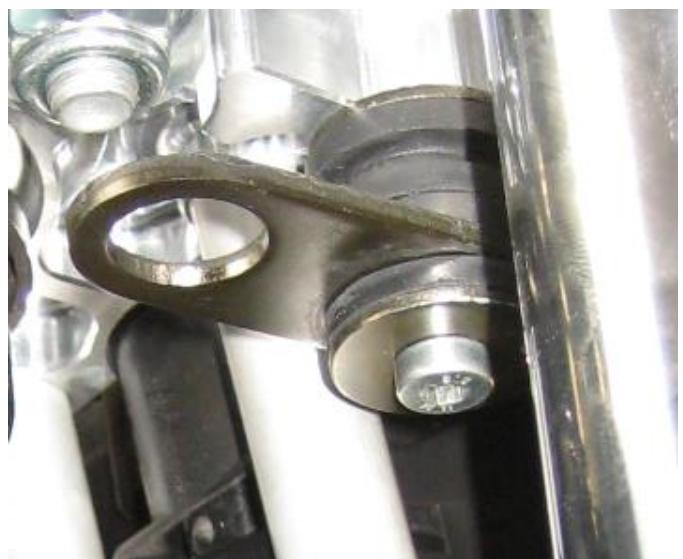
4. If the original fender is used it must be installed with 4 spacers (5), bolts (12) and washers (8).
