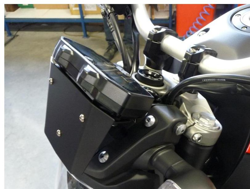
**05.** Now connect the wiring harness and move the speedometer in the already mounted LSL speedometer bracket and fix the speedometer with the original screws.
