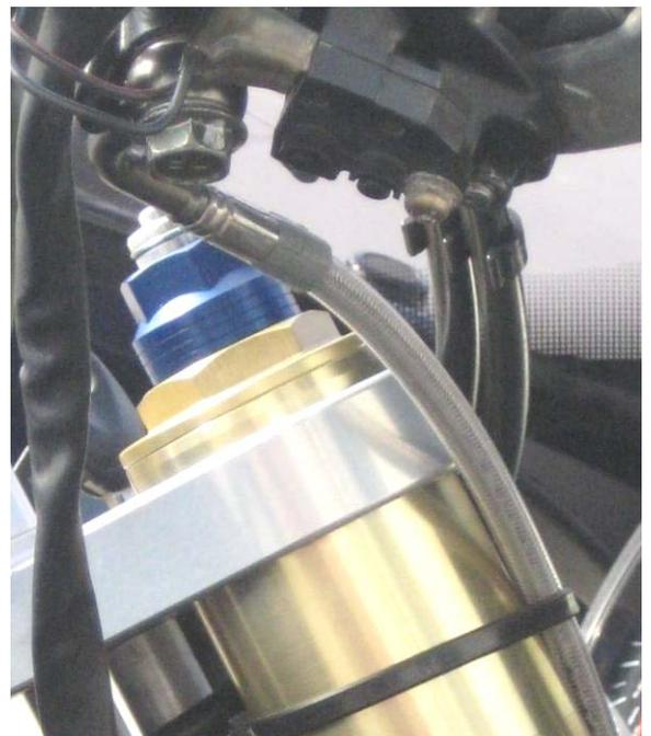
**Clutch cable (3):** Route clutch cable as shown and protect it, with the attached shrink hose, from chafing on the marked spot (see →).
