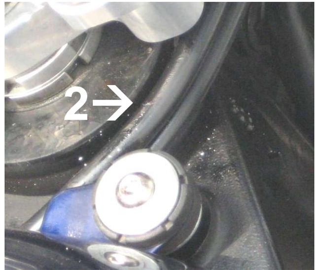
**Brake hose (2):** Fit the attached hose with new seal-rings. Mind the mounting instructions that are delivered with the brake hose. Mount the brake hose (79cm) with 90 degree sideward bended fitting on the brake cylinder as shown and fix it with a cable tie at the slider-tube. Route hose as original through the guidance at the bottom yoke.
