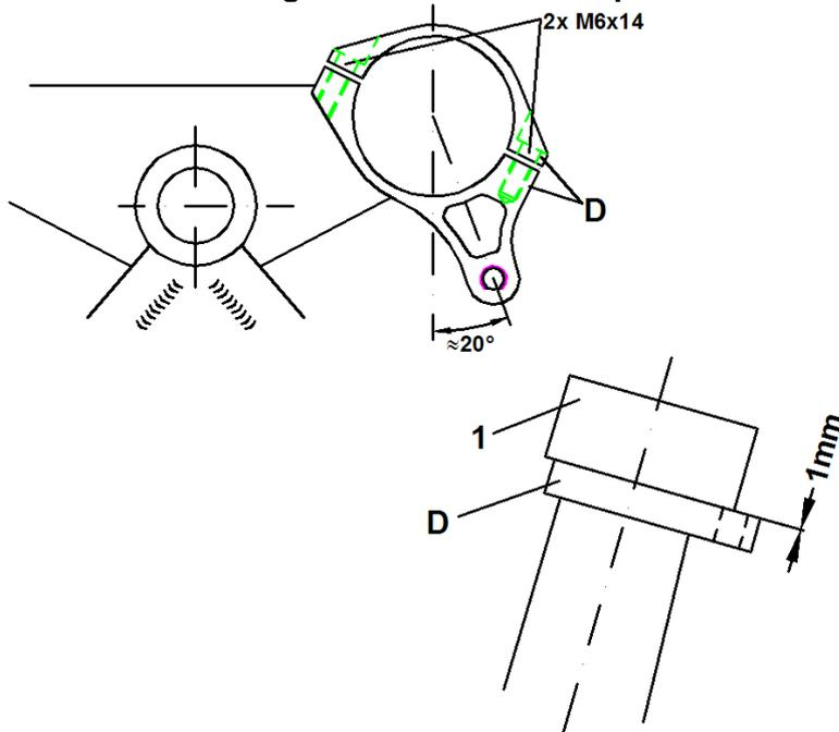
3. Mount the clamp (D) with screws M6x14 on the slider tube, underneath the top yoke (1). Adjust it as shown but do not tighten it too strong, so it may be necessary to adjust the damper by turning the clamp slightly.
